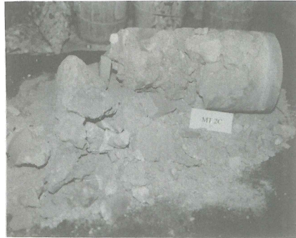
Fig. 14 - MTc sample after failure
