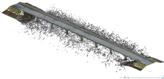
Figure 3. Original point cloud data with significant quantities of noise in evidence
