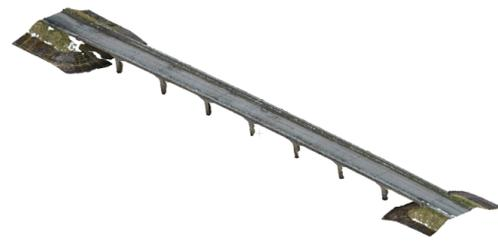
b. Point cloud after automatic noise removal
