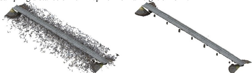
Fig. 3. a) A point cloud of the bridge from a image acquired from UAV b) A point cloud after removing noise data
