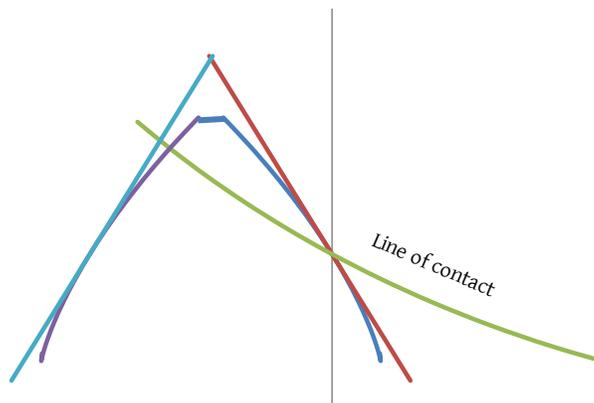
Figure 10. The triangular tooth profile, the line of contact, and the profile that is conjugate to the triangle.
