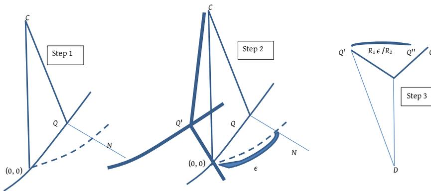
Figure 2. Steps in the construction of the point  $Q''$  (on the gear  $D$ ) which is conjugate to  $Q$  (on gear  $C$ ).
