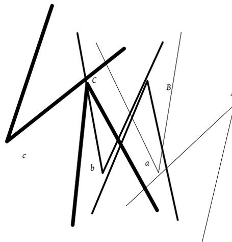
Figure 6. The discontinuity in rotation rates occurs as the gears pass through configuration  $Bb$ . The line of contact is  $abBCa$ . It comprises two circular arcs,  $ab$  and  $BC$ , and two discontinuous jumps,  $bB$  and  $Ca$ .
