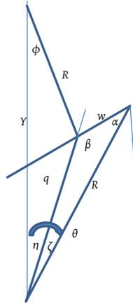
Figure 4. Quantities used to determine the rotation of two gears with triangular teeth.  $Y$  is the line joining the centers of the gears.  $R$  is the radius vector to the tip of a tooth on the upper gear.
