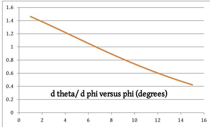
Figure 5. Showing the variation in  $d\theta/d\phi$  as a single tip slides over a single face.
