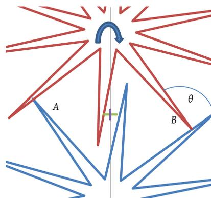
Figure 8. The gears jam when the pressure angle  $\theta$  exceeds  $\text{atan}(1/\lambda)$ .
