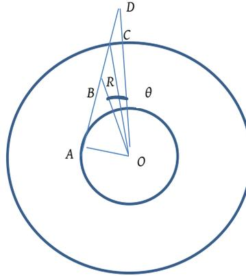
Figure 9. The sides of a triangular tooth are tangent to a circle  $OA < OC$ .
