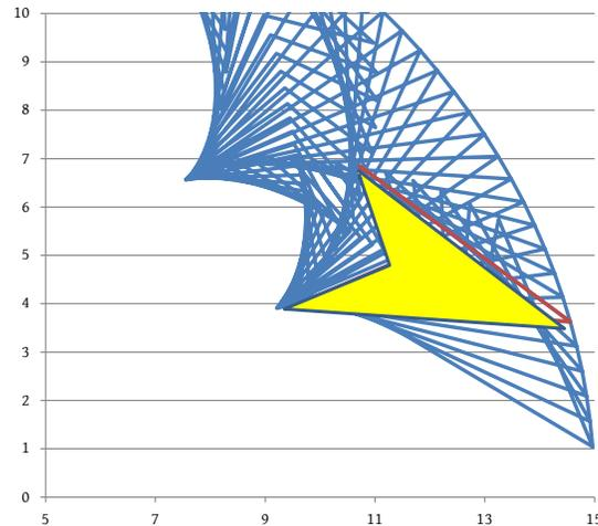
Figure 11. A gear with triangular teeth, only a slice of which is seen here, is rolled around a fixed circular gear blank, cutting away, as it goes, any material that gets in its way. What remains is the conjugate tooth shape conjugate to the triangle. Compare to the conjugate shape determined by analysis in figure 10.
