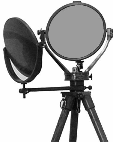
Figure 1. The optical telegraph.
