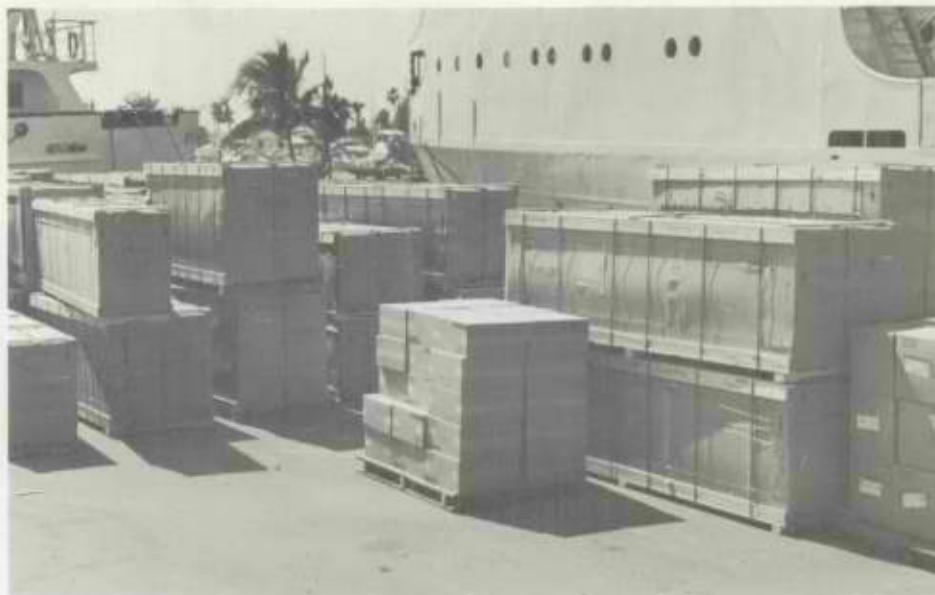
"The Motel That Went To Sea" — 150 crates of containerized pre-engineered Panelfab motel rooms were shipped to the Island of Grenada for expanded guest facilities during a trade exposition.
