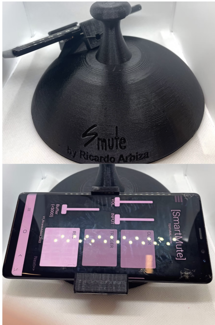
Figure 19: Smute: 3D-printed plunger mute with integrated smartphone interface.
