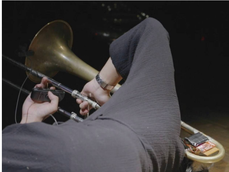
Figure 17: Mubone: Joy-Con controller and orientation sensor on the fine-tuning slide (West and Leung, 2022, p. 9)
