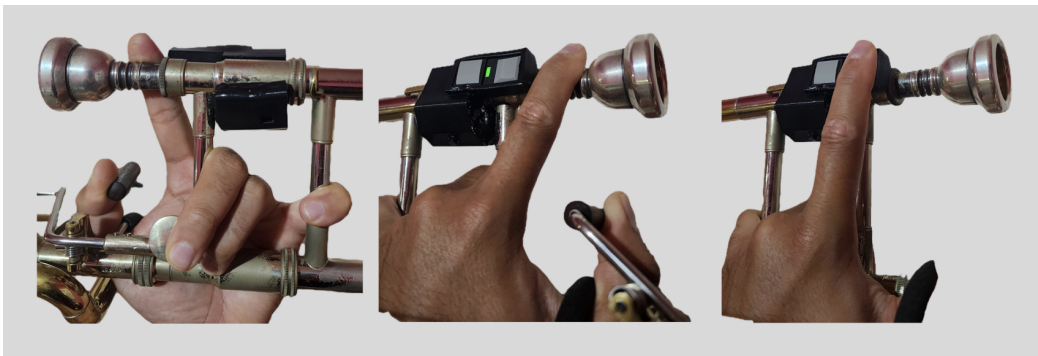
Figure 89: Evolution of the second prototype 3D-printed housing with different designs and materials
