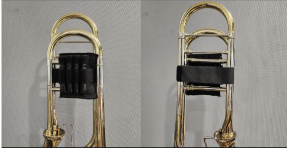
Figure 28: Incremental weight pouch mounted on the back of the F-attachment trombone, shown from front and reverse angles.
