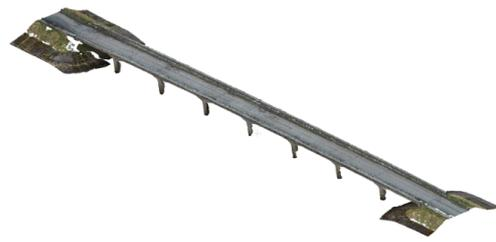
b. Point cloud after automatic noise removal
